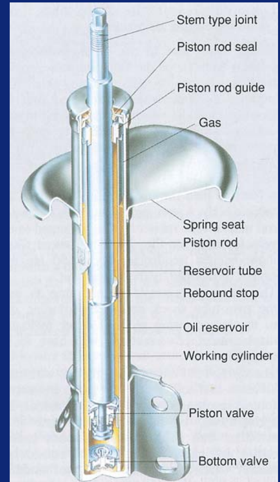
Design of a twin tube spring strut
